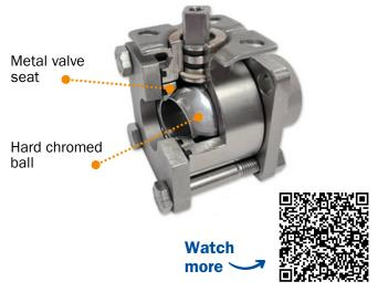
Jouka metal seated valve materials are stainless steel 316L, 304L, and Duplex – as well as carbon steel. Their simple construction and carbide coated seat ensure a long lifecycle.
